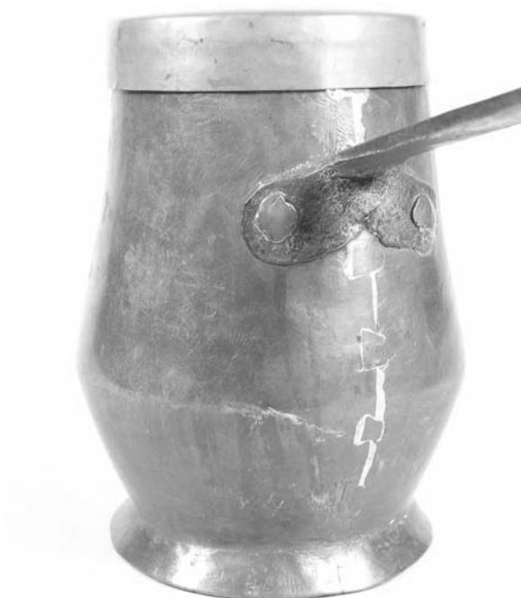
FIGURE 54.4. Chocolate pot construction: example of simple flange handle. Source: Courtesy of Christopher D. Fox. (Used with permission.)
