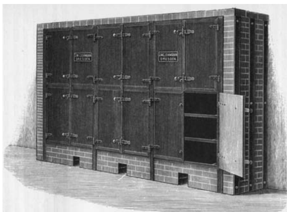
FIGURE 46.5. Holding room for chocolate liquor. Source: Paul Zipperer, The Manufacture of Chocolate , 2nd edition, 1902; p. 143. Courtesy of Rodney Snyder. (Used with permission.)
